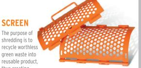
thus creating added value. Material is often a decisive factor for potential applications. The Mega Prof allows you to adjust this. Thanks to the calibration screen, you can control how long the chips stay in the chipping chamber, and thus also how finely they are cut.
