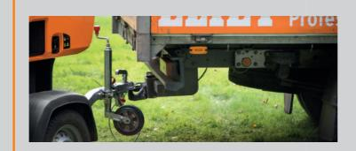
The chassis is a sturdy, fully welded and galvanized frame. This rigid frame rests on a spring-loaded axle with a wheelbase of 180 cm. In combination with a low center of gravity, this provides excellent road holding. The trailer is fitted with a height-adjustable support wheel and two extendable support legs that enable stable setup once unhitched. It comes standard with chocks.
