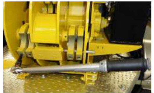
Screwlock knives and hammers: 157 N.m.
