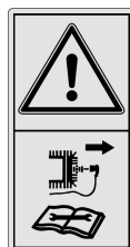
Switch off the engine and remove the spark plug cap before repair, maintenance and cleaning!
