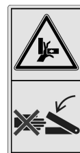
Never reach into the crushing danger zone if parts can still move there!
