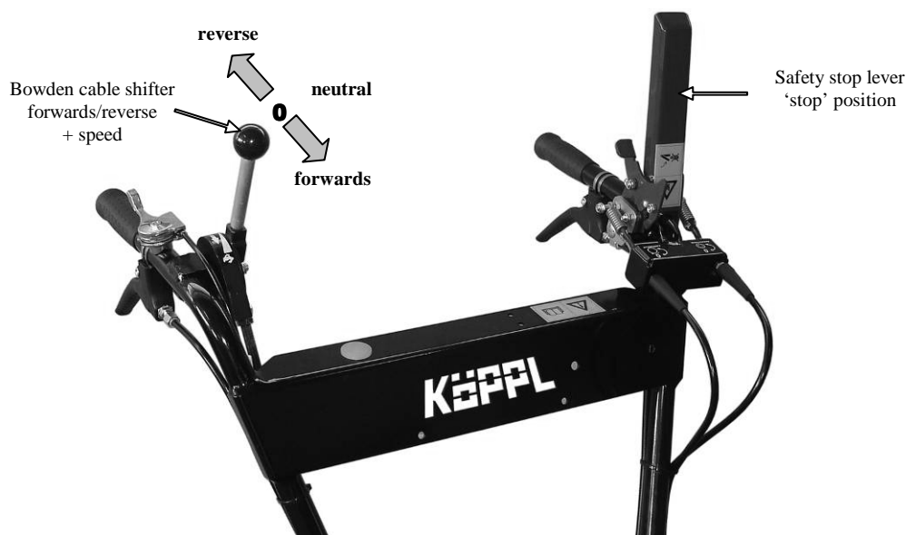
Fig. 2. Safety stop lever – stop position.
