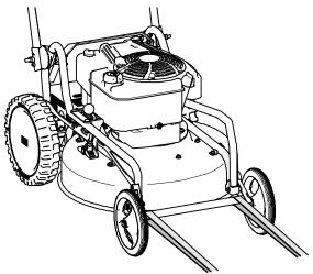
Use tension belts to secure the device.
