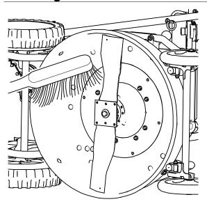
After each use, you should clean the device thoroughly, especially the bottom side and the blade.
